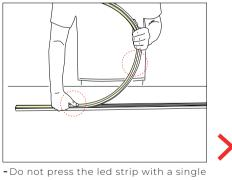
Do not press the led strip with a single finger, it is easy to damage the internal
