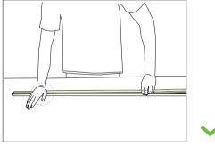
Please press the led strip with your palm to slowly insert the led strip into the groove, and gently straighten the led strip above the groove with your right hand.
