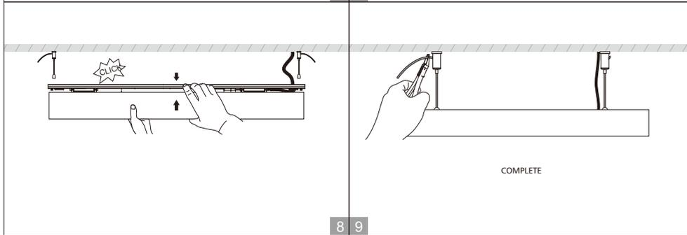
Suspended Installation (With round ceiling plate)
