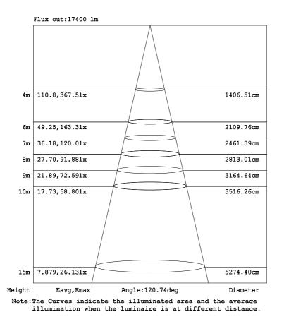
C Range: 0 - 360DEG C Interval: 22.5DEG Test Speed: HIGH Temperature:25.3°C Operators:WJH Test Date:2023-08-05
