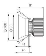
**LED Chip UGR** Citizen COB <19 Life Expectancy Efficacy 40,000 hrs TM-21 Up to 98lm/W **SCDM LED Driver** <3 Macadam steps</p> Dimmable Connection **Working Temp** -20°C to +45°C LED Driver, Lead & Plug **Power Factor** Tilt Angle ≥0.9 36° Carton Qty CRI 24 ≥80
