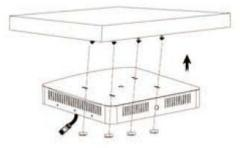
Place the cover on the ceiling and mark out the 4 screw holes. Then remove the cover and drill the 4 holes. Place the cover on the ceiling, lining up the 4 holes and screw the cover to the ceiling. Then connect the driver to the lamp.
