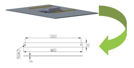
Step 4: Finally fix it to the plate using 4 M6 screws.
