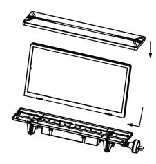
3. Connect the battery to PCB and securely attach the fixture onto the ceiling.
