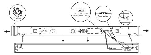
Step 2: Mount the fitting onto ceiling with wall plugs and screws
