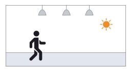
1. When the ambient light is bright enough, the light will not automatically light up even if a moving object is detected.
