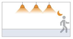
3. After the moving object leaves, the sensor will enter the delay time when it cannot detect the moving object and keep the light on.
