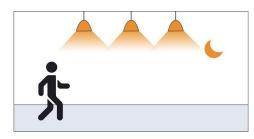
2. When the ambient light is lower than the preset photosensitive threshold, the light will automatically light up when the sensor detects a moving object.
