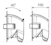
LED Chip Efficacy Citizen COB Up to 121lm/W Life Expectancy **LED Driver** Dimmable 40,000 hrs TM-21 Working Temp Tilt -20°C to +45°C From 24° up to 45° CRI Connection >80 LED Driver & 600mm Lead **Power Factor** Carton Qty
