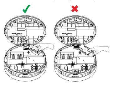
**3.** Insert the battery into the slot. Ensure the right side of positive and negative pole.
