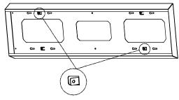
3. Pull up the corners of the surface mount kit for the safety cables.
