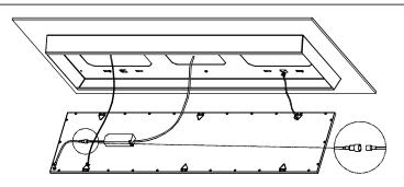
7. Securely attach the safety cable to the LED Panel.
