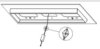
5. Connect the power supply to the electricity supply.
