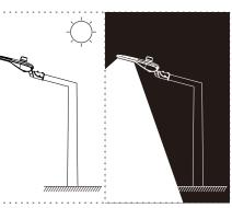
Note: If the luminaire use 5 pin or 7 pin photocell socket, it need to plus a waterproof gasket between socket and photocell controller.
